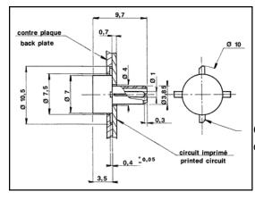
Corner cut indicates center pins (positive) Weight : 0.71gr
